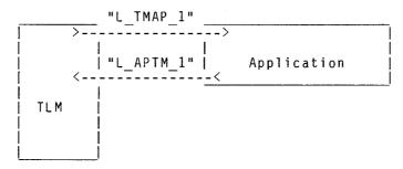
The request sent contains enough information for TLM to initialise the required TLink services. Once TLM has initialised the TLink entities it will send a TLM\_SERVICE.response (s. 4.2.1.1.1) to the Application through pipe "L\_TMAP\_1". The information contained in the response will indicate to the application whether its request was successful or not.
