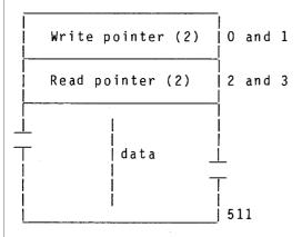
The physical layer updates the write pointer when data is put into the buffer. The read pointer is never changed by the physical layer. The physical layer writes data cyclically and makes no attempt to check wrap-around. It is recommended that changes to the write pointer, other than by the physical layer, are done with caution.
