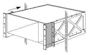
**b** Insert the two middle fasteners (screws).
