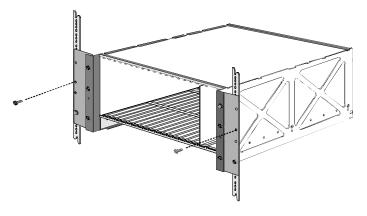
c Insert the two top fasteners (screws).
