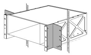
**b** Insert the two middle fasteners (screws).
