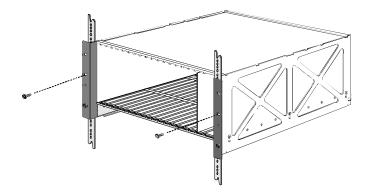
**b** Insert the two middle fasteners (screws).
