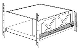
**4** Secure the bracket to the chassis.
