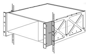
c Insert the two top fasteners (screws).
