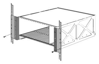
**b** Insert the two middle fasteners (screws).
