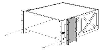
**b** Insert the two middle fasteners (screws).
