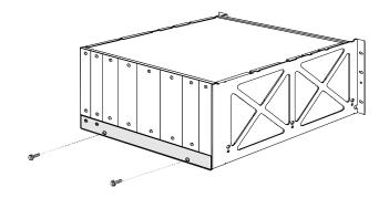
**2** Loosen the two fan tray screws at the front of the chassis.
