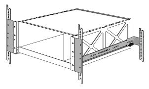
**4** Secure the bracket to the chassis.
