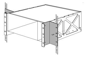
**c** Insert the two top fasteners (screws).
