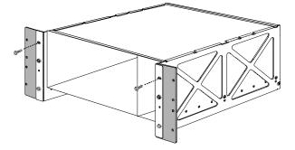
**3** Slide the chassis into the rack, until the front of the chassis is flush with the front of the rack.
