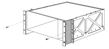
**c** Insert the two top fasteners (screws).
