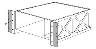
c Insert the two top fasteners (screws).
