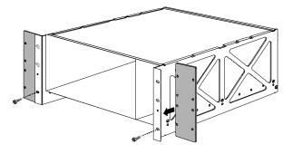
**b** Insert the two middle fasteners (screws).
