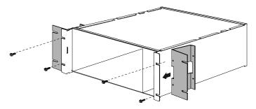
2 Slide the chassis into the rack, until the front of the chassis is flush with the front of the rack.
