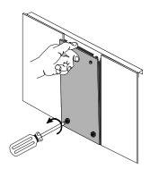
**5** Install the NAC in the appropriate slot in the chassis.
