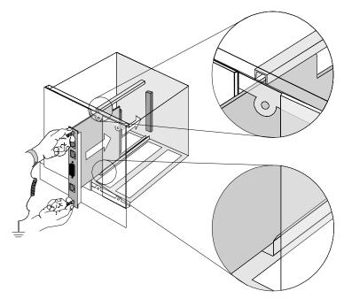
4 Slide the NIC into the chassis, until the front of the NIC is flush with the chassis.
