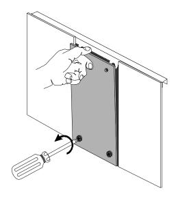
3 Insert the NIC between the slot's upper and lower card guides.
