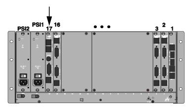
**2** Use a #2 Phillips screwdriver to remove the safety panel covering this slot.
