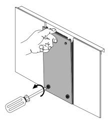
**5** Insert the NAC between the slot's upper and lower card guides.
