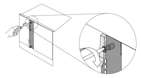
7 Use a flat-head screwdriver to tighten the screws on the front panel.
