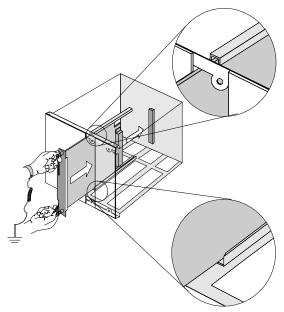
6 Holding the tabs perpendicular to the NAC's front panel, slide the NAC into the chassis, until the front of the NAC is flush with the chassis. Push the tabs toward each other to secure the NAC.
