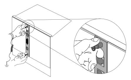
Use a flat-head screwdriver to tighten the screws on the front panel.
