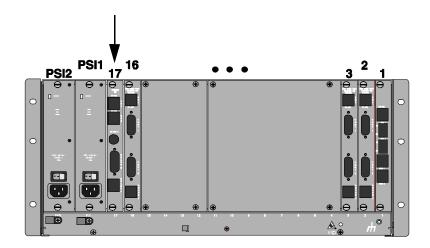
**3** Use a #2 Phillips screwdriver to remove the safety panel covering this slot.
