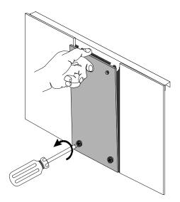
4 Insert the NIC between the slot's upper and lower card guides.
