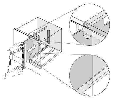
**5** Slide the NIC into the chassis, until the front of the NIC is flush with the chassis.
