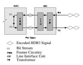
Configure the NAC framer to respond or ignore the loop-up/loop-down pattern from the Telco.
