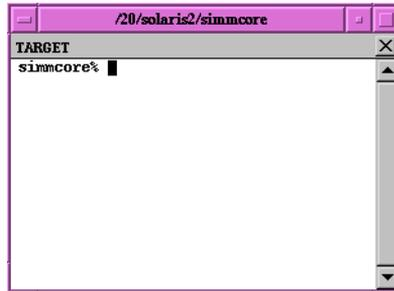
2. The **I/O Window** provides **stdin/stdout** to the target. For example, when **printf** is called from the target, the output is displayed in this window. This window works with the standard ANSI IO libraries provided by GHS. If you have your own IO routines, the debug server IO window is ignored.
