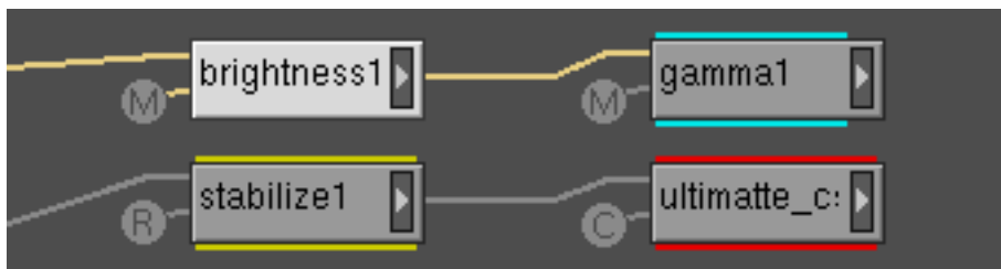
5.14 Node feedback, clockwise from top left: Brightness is selected; Gamma is pinned to a view; Stabilize is in alert mode; Ultimatte CSC is in error mode (because it requires the other input to be connected).
