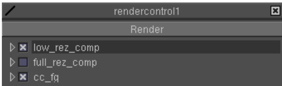
11.1 Render Control View: the “full_rez_comp” entry has been disabled, as checkbox next to entry name indicates; “low_rez_comp” is selected, as indicated by shading.
