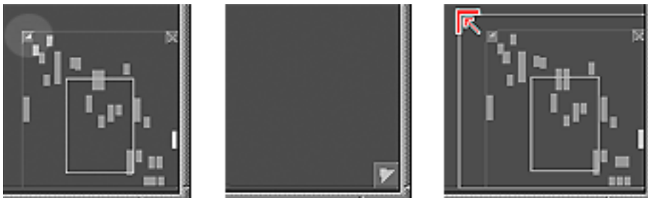
5.2 Navigator: Click button (highlighted, left) to stow (middle); drag button to resize (right).
