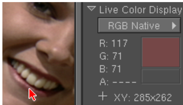
6.6 Live Color Display shows the RGBA values and x,y position of the pixel under the cursor.
