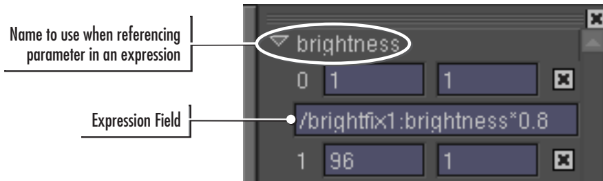
C.3 Expression field for a key-point in the Keypoint Viewer panel of the Curve Editor.
